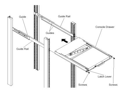
Installing the Console Drawer diagram
