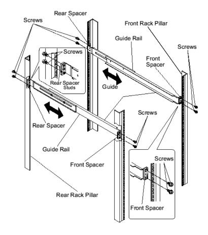
Installing the Guide Rails diagram
