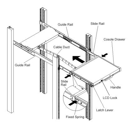
Inserting the slide module diagram
