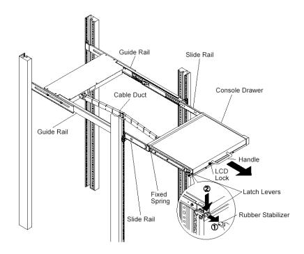
Pulling out the slide module diagram
