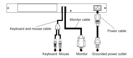
Connecting cables to Console Drawer diagram
